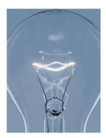
Fig. 14.12 Glowing filament of an electric bulb
