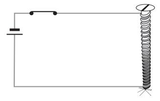
Fig. 14.19 An electromagnet
