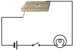
**Fig. 14.17** Effect of current on a compass needle
