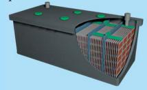
Fig. 14.6 Truck battery and its cutout
