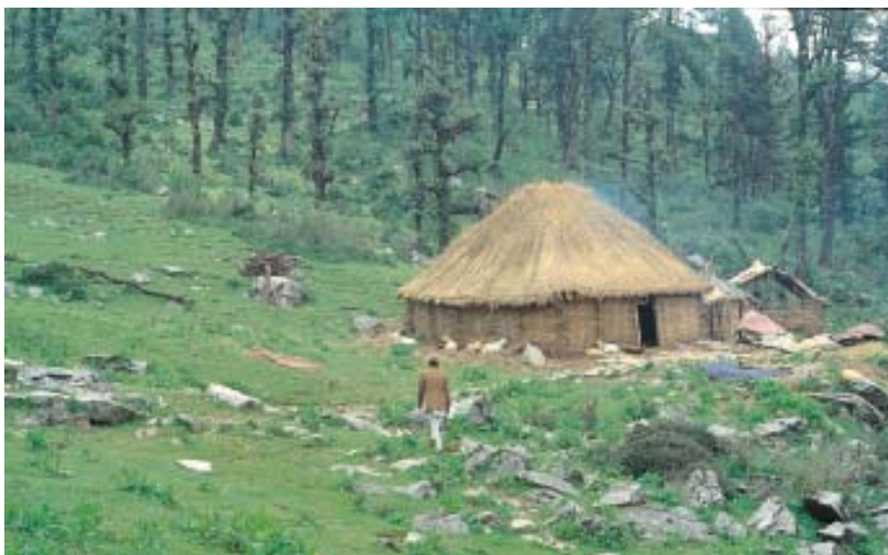
Fig.2 – A Gujjar Mandap on the high mountains in central Garhwal. The Gujjar cattle herders live in these mandaps made of ringal – a hill bamboo – and grass from the Bugyal. A mandap was also a work place. Here the Gujjar used to make ghee which they took down for sale. In recent years they have begun to transport the milk directly in buses and trucks. These mandaps are at about 10,000 to 11,000 feet. Buffaloes cannot climb any higher.
